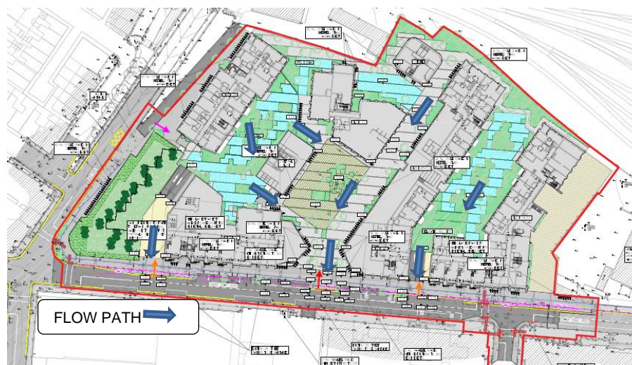
Figure 5-2: Overland flow path
