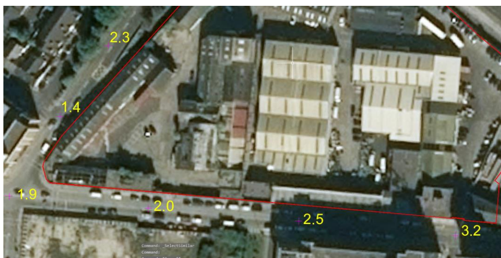
Figure 5-1: Existing road and boundary levels in the vicinity of the proposed development site
